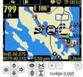
This screen contains a number of buttons for adjusting the coordinates of the map. As well, a nudge factor can be set for adjusting the precision to which to move the map.
