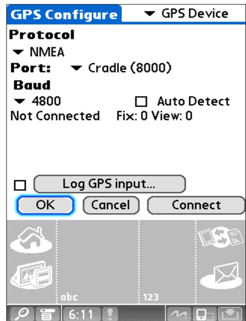
The most common baud rate for most GPS devices is 4800 BPS. Next is 9600, followed by 57,600.
